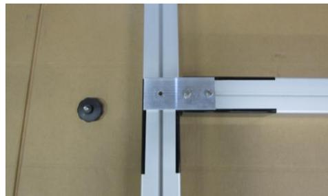
Fix additional bar with hand wheels (see pictures bottom left and right). Then tighten hexagon socket screws already mounted at the bar (see picture bottom right). Finally fix again removed or unscrewed parts at the bottom of uprights.
