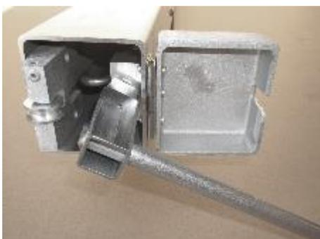
Open the cap at the mechanical upright and set the square key wrench on the spigot of the spindle. Now pull up the provided hook by turning the wrench.
