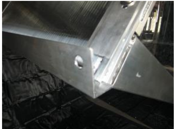
Picture 25 + 26: Fix angles 50x30x2mm at roof cross brace and side parts with pan head screws DIN 85 M6x20 and washers DIN 9021 Ø 7.4 mm. Now all screws should be tightened.
