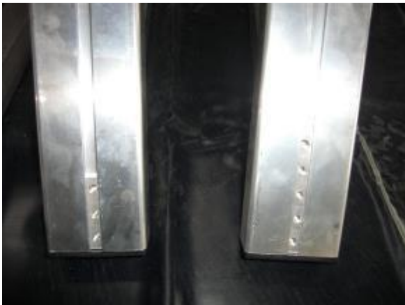
Picture 29: Stick plastic caps on middle supports. Push at first 4 nuts M6x20 in the 2 exterior middle supports, then 1 nut M8x20. Push 2 nuts M6x20 and 1 nut M8x20 in the remaining middle supports (2-4 according to cabin width).
