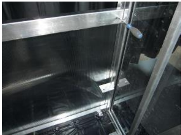
Picture 12: Connect side parts and rear wall with pan head screws DIN 7380 M8x16. Remove protection foil of side part.
