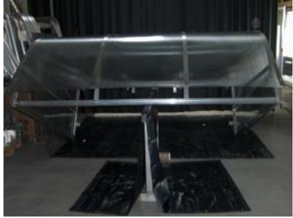
Picture 24: Turn over the cabin and adjust nuts which were pushed in the roof cross brace (see picture 15) in front of the middle supports.
