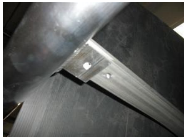
Picture 18: Screw other side of roof middle supports at welded plates of roof cross brace using rounded head screws DIN 7380 M8x16.
