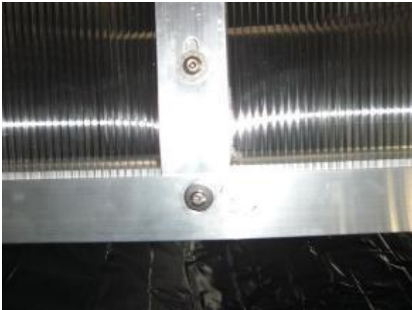
Picture 25 + 26: Fix angles 50x30x2mm at roof cross brace and side parts with pan head screws DIN 85 M6x20 and washers DIN 9021 Ø 7.4 mm. Now all screws should be tightened.
