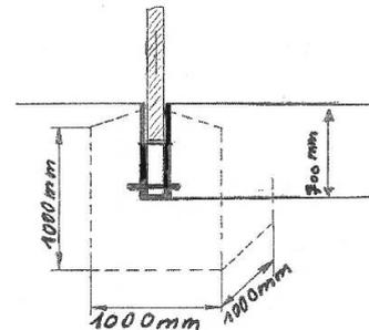
1. Fix ground sockets **“for plugging”** on concrete foundation corresponding to the playground size. Consider that the ground sockets are made with a negative-going inclination of 1°. “Number 1” is stamped on the ground plate of the ground socket which has to point to the inside towards the net during plugging.
