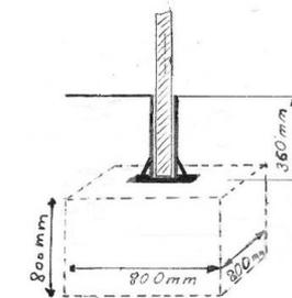
2. Fix ground sockets **“for concretion”** corresponding to the playground size. We recommend to place them negative-going by about 1° inclination to the outside.
