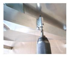
A sleeve with thread M8 is welded on one of the reel supports. Bore a hole for the lock through the sleeve with drill  $\emptyset$  9.5 mm at any position in the round side part.
