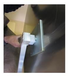
To insert the reel press both side parts outwards and push polyamide liners into the square attachments. One side part is equipped with a welded sleeve to lock the reel later.
