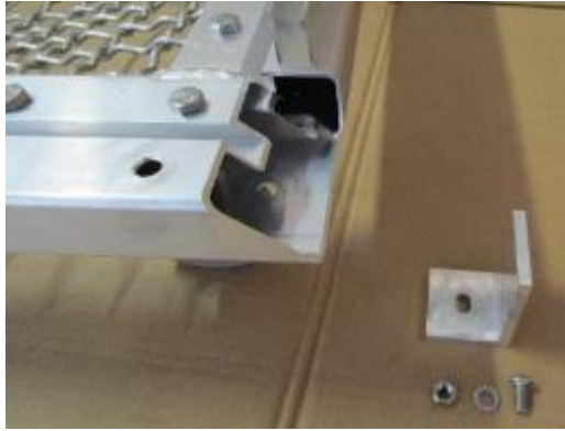
Fixing of angle 75 x 50 x 7 mm, length 50 mm at the back of the bottom part
