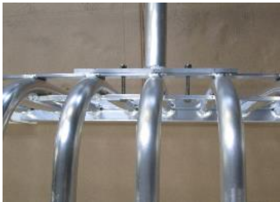
plate of brace: adjust holes and holes of flat profiles of the goal congruently
