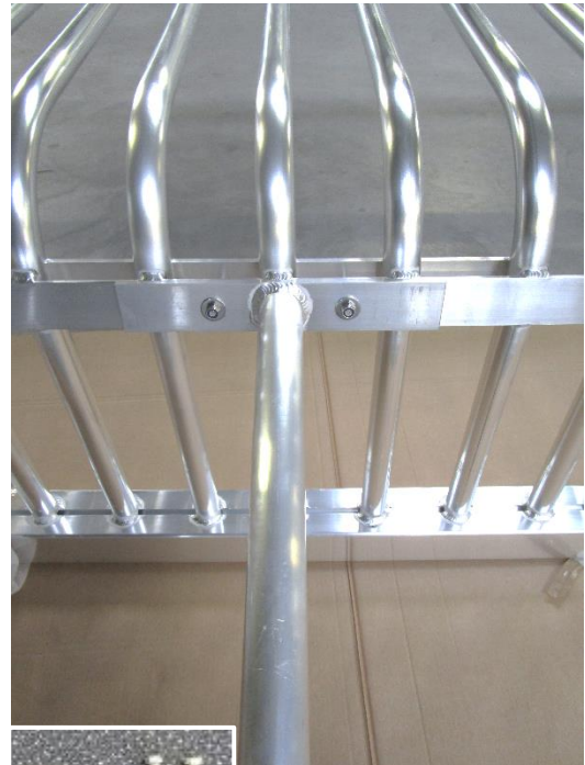
plate of brace: adjust holes and holes of flat profiles of the goal congruently
