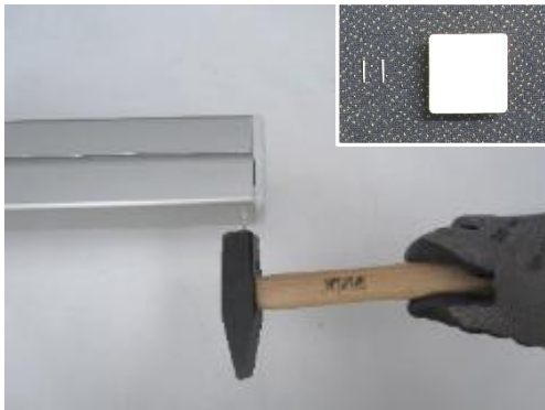
Fixing of cap in square upright:
