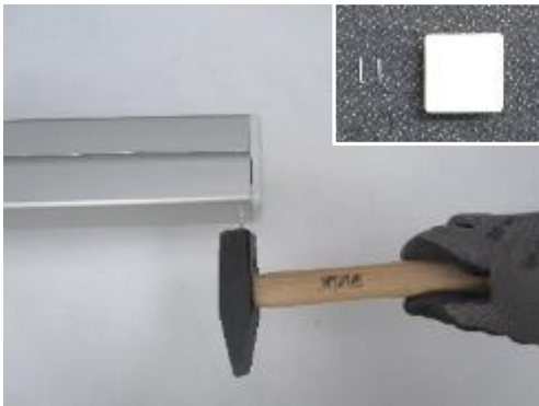
Fixing of cap in square upright:
